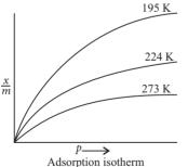
These curves indicate that on increasing temperature, physical adsorption decreases at a fixed pressure.
